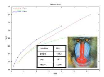
Figure 4: BTPC's worst case out of a test set of 80 standard photographic images. For this highly-textured colour image, BTPC 5 is also worse than BTPC 4.1 at low data rates! This is the only such case and illustrates where the assumption of local colour dependence fails.
