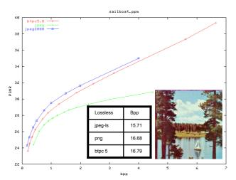
Figure 3: A representative example of coding a photographic image. In most cases BTPC 5's performance is inferior to JPEG2000, but the gap between BTPC and JPEG2000 has been closed by the exploitation of colour dependencies in version 5. For lossless coding of photographs BTPC uses 0-10% more bits than JPEG-LS.
