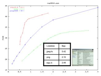
Figure 5: A representative example of coding a graphical/textual image, in this case a screen shot. Sometimes worse than PNG for lossless coding, BTPC's lossy coding causes little visible distortion even at half the PNG data rate. BTPC always outperforms the lossy alternatives, usually by a significant amount.
