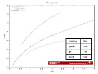
Figure 6: BTPC's worst case out of a test set of 40 graphical images relative to the better of PNG and GIF. GIF performs best on small, palettized, highly-structured images. In such cases, lossy BTPC coding at the rate achieved by GIF produces very good graphics
